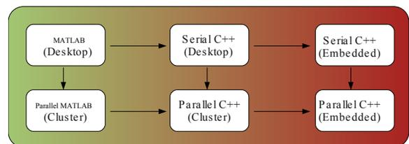
Figure 11. Integrated development workflow from prototyping to deployment, using MATLAB and Sourcery VSIPL++
