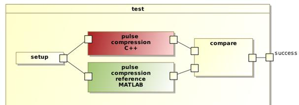
Figure 9. Testing of the new C++ implementation against the gold standard
