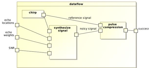
Figure 6. Composite structure of a test application for the pulse compression algorithm
