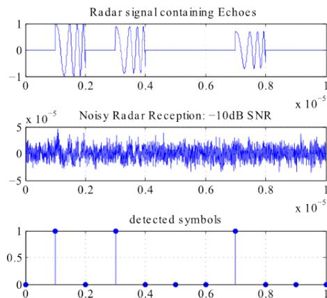
Figure 3. Pulse compression simulation results for -10dB SNR
