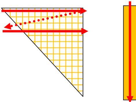
Figure 2: R Matrix and  $Q^*b$  sample calculation order
