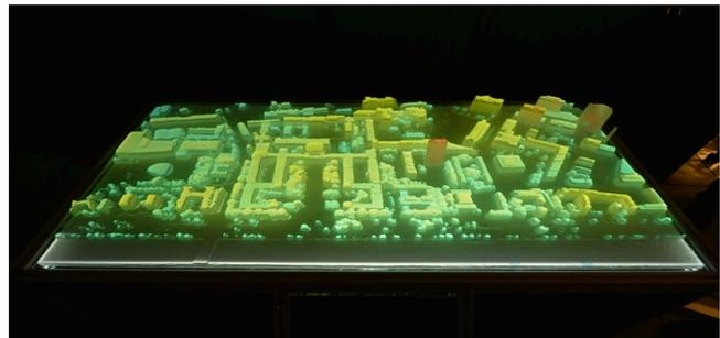
Fig. 1. (a) LuminoCity with Projector Base (b) LuminoCity illuminated by measured height above ground level (data generated by LADAR)
