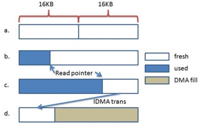
Fig. 1: (a) the logical organization of the buffer, (b) buffer state before the accumulation loop, (c) buffer state after the accumulation loop, (d) IDMA and DMA transfers performed.
